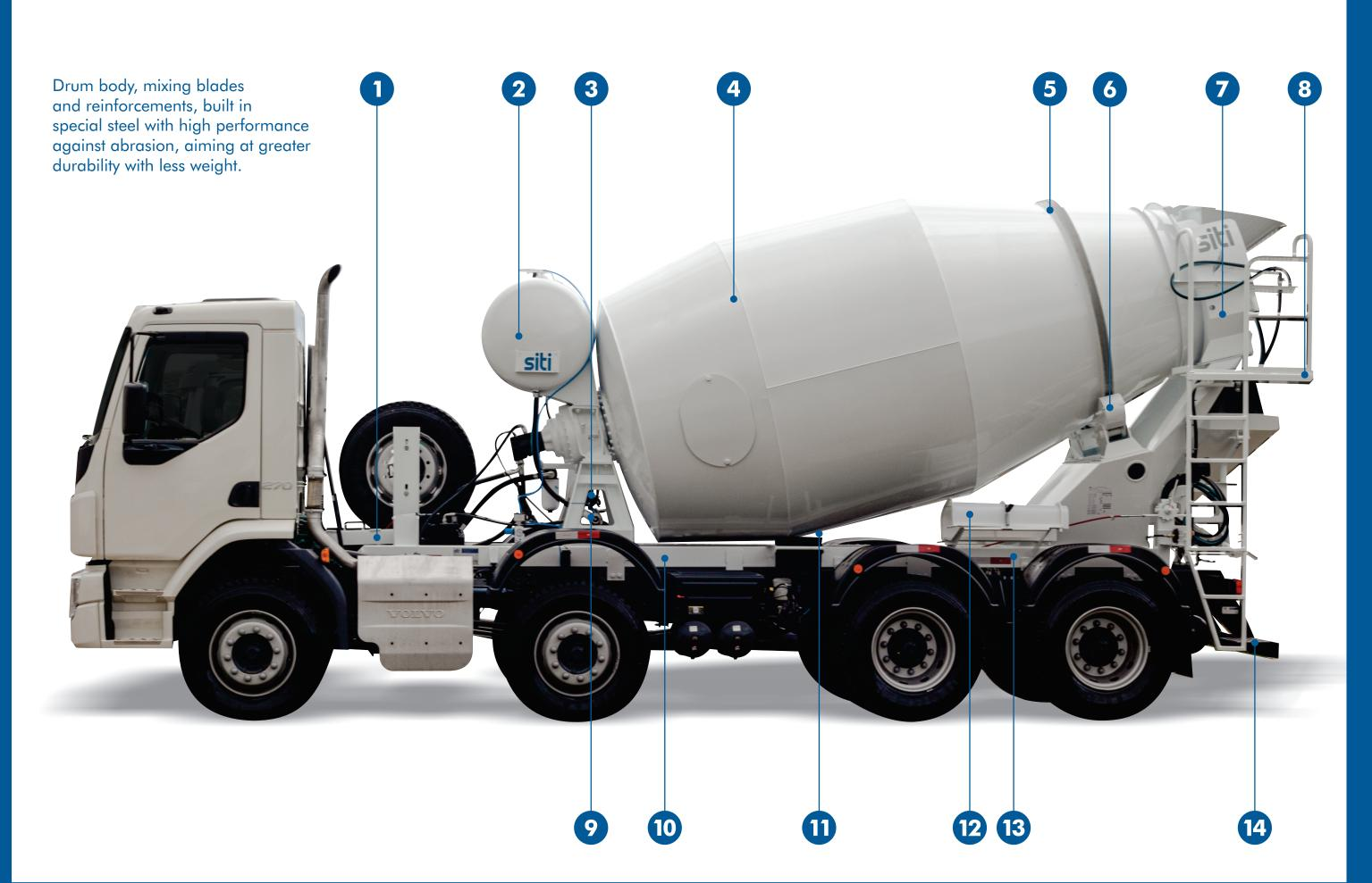
Ladder with non-slip steps and expanded sheet metal platform, which is also easier to clean.
