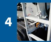
Ladder with non-slip steps and expanded sheet metal platform, which is also easier to clean.
