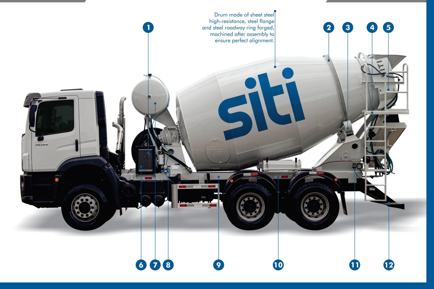
Reservoir with capacity for 600 liters of water, pressurized with 5 kg/cm², with safety valve, water volume register by hydrometer with reading from 0 to 500 liters and hose for
