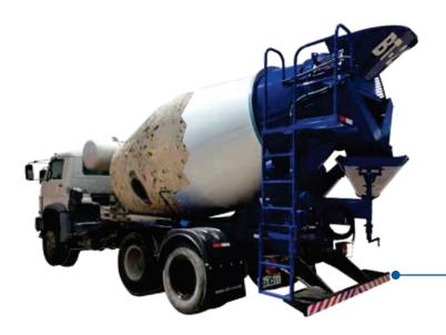
With more than 30 years of experience in the concrete mixer market, we guarantee a quality renovation. Our restoration process includes steel shot blast preparation, which removes practically 100% of the impurities on the sheet surface and increases the durability of the painting.
