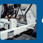
Chassis manufactured in a single piece, avoiding assemblies and screws, adding greater stability to the equipment.
